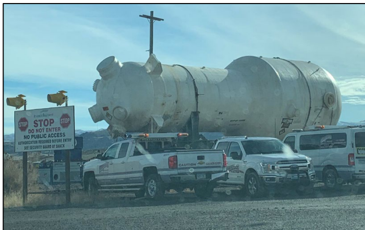
Arrival of a steam generator at EnergySolutions' large component cell
